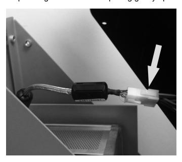
Figure 4 - LED cable harness connector
