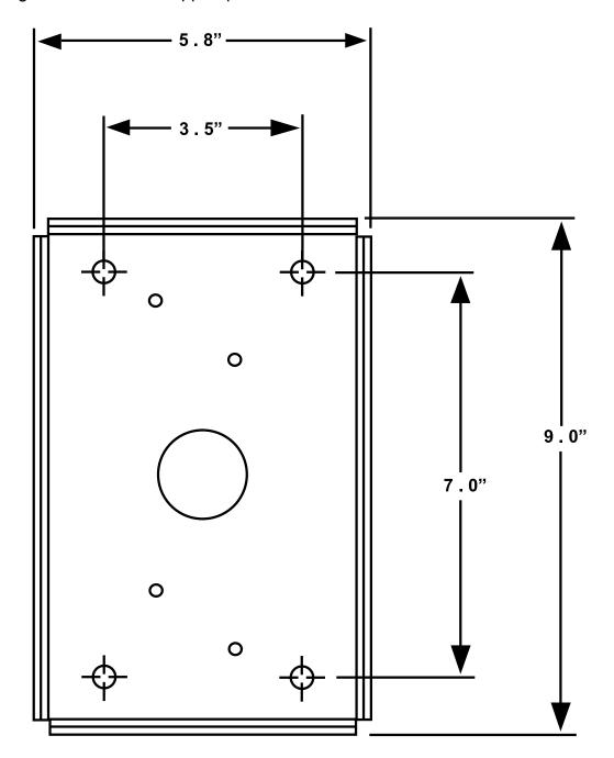
Figure 1 – L1 PowerPost™ EVSE Footprint & Mounting Hole Locations
